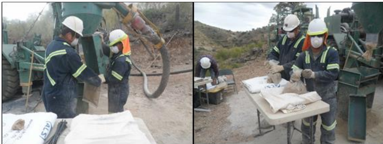
Figure 11:1 Cerro Caliche Project, RC Drilling and Sampling Procedure
